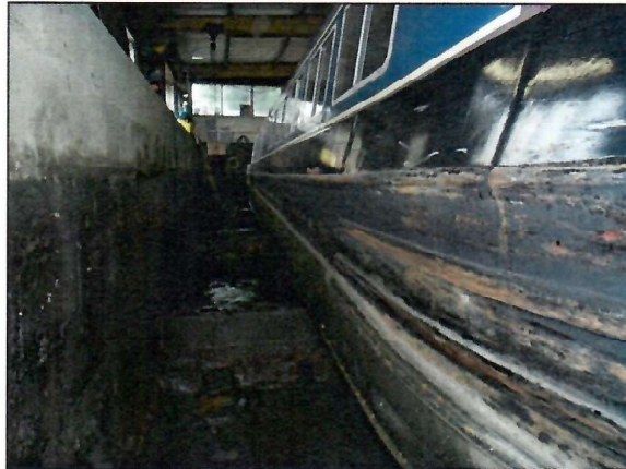
Hull sides showing scuff marking.
