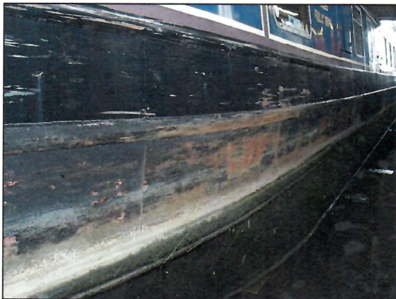
Hull sides showing scuff marking.
