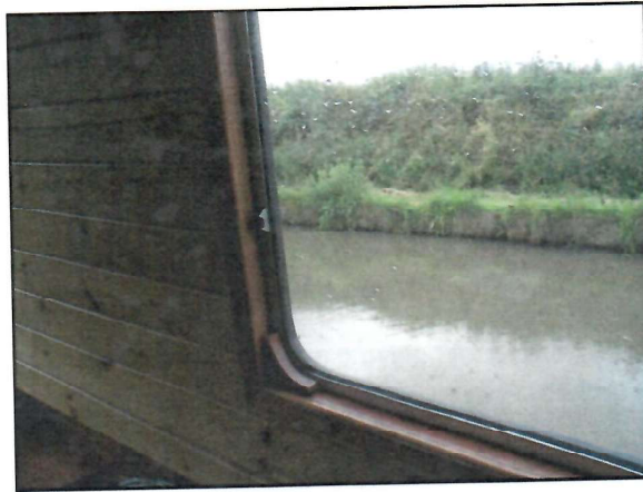
Cabin window – note the missing catch.
